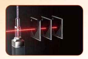
H80 series hematology analyzers utilize the semi-conductor laser technology for WBC differentiation. 3 different angle scatters reflect information of the cells in an all-round way.
